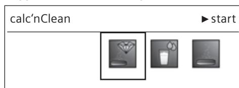
The **start** button **8** flashes while the different calc'nClean processes are running. The figures on the top right indicate the progress of the programme.
