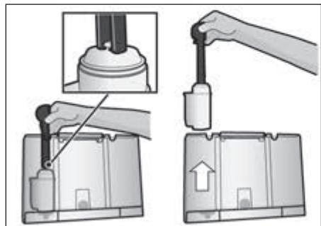
**Info:** Rinsing the filter **29** simultaneously activates the setting for the "change filter" display.
