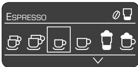
The status line **5a** in the display shows the name of the type of drink, along with the strength setting, e.g.  $\emptyset\emptyset$  and per-cup quantity, e.g.  $\square$ . The selection line **5b** shows symbols for the drink selection. The arrows in the navigation line **5c** indicate the direction in which more menu levels can be found.
